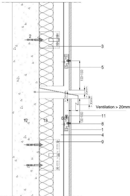
**Figure 26 - Splitting the framework: Aluminium posts between 3m and 6m in length**
