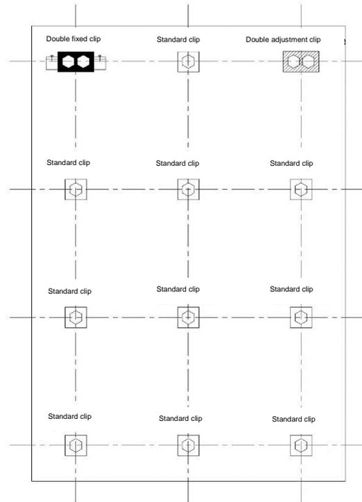
**Figure 7 - Positioning clip types**
