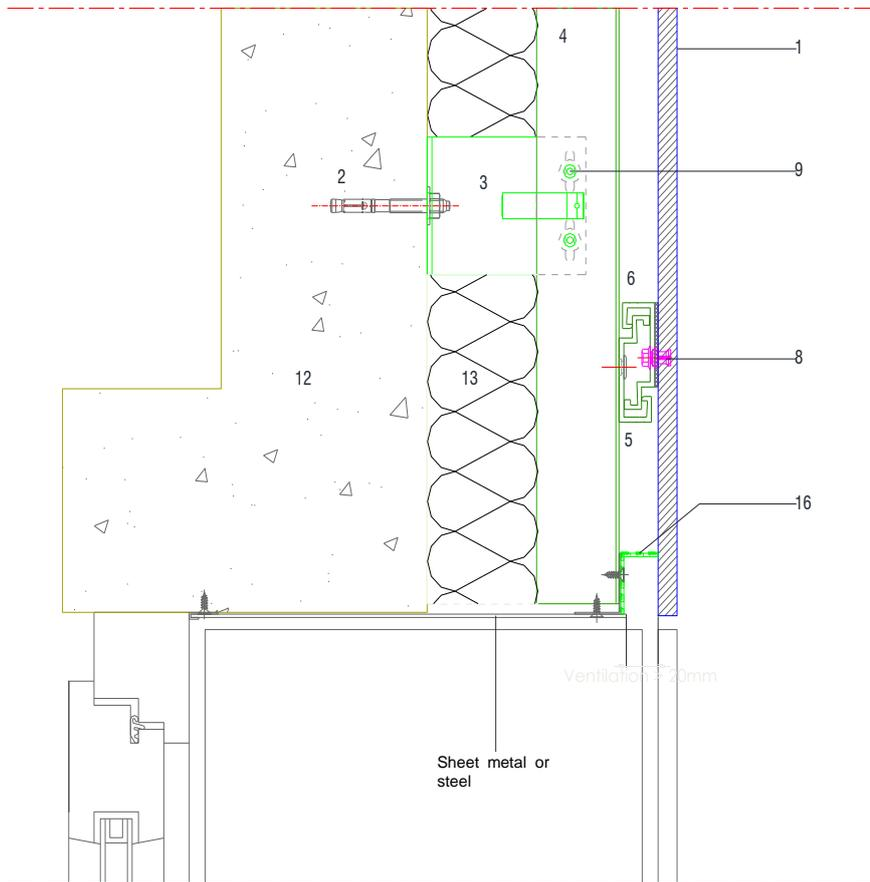
**Figure 19 - Window lintel with sheet metal cladding**
