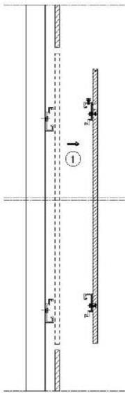
Cut 2cm from the panel and remove the panel.
