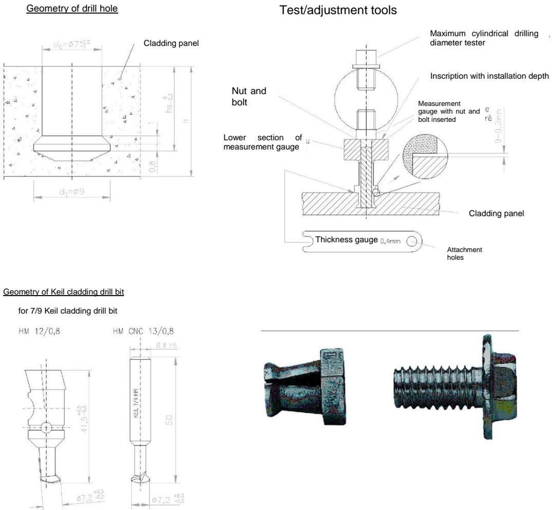
Figure 3a - Geometry of KEIL-1
