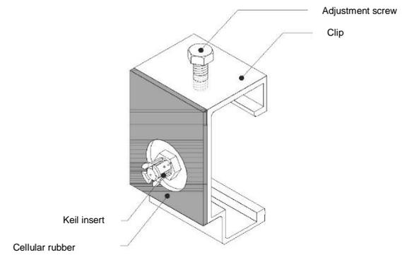
Installing the adjustment clip
