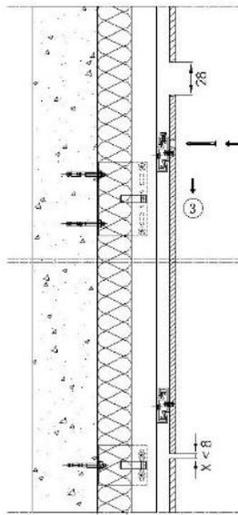
Lower the replacement part until the clip locks into the rail.
