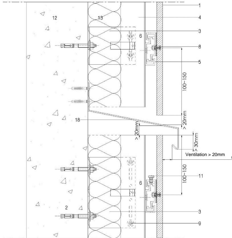
**Figure 15 - Horizontal compartmentalisation of air gap**
