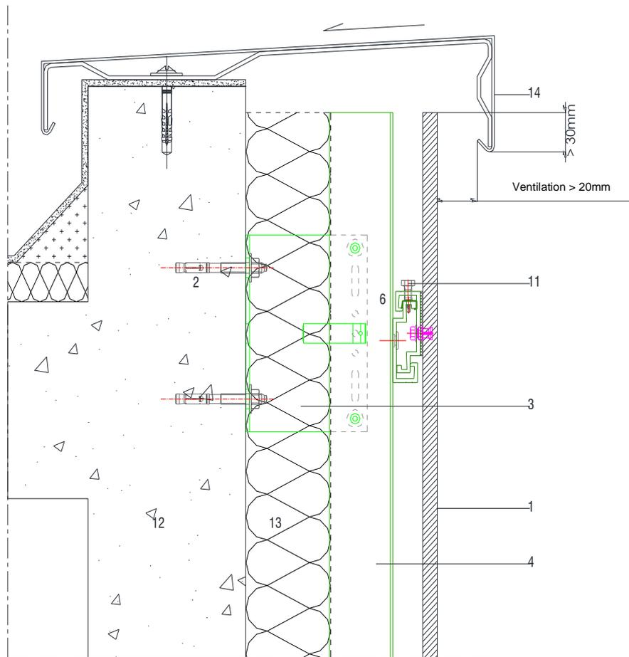
**Figure 13 - Parapet cap**
