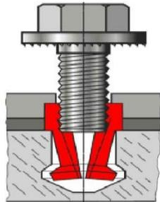
a) Insert the sleeve in the hole and drill the screw in the sleeve
