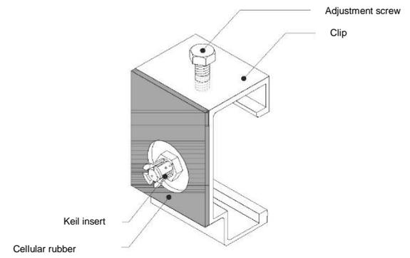
Installing the adjustment clip
