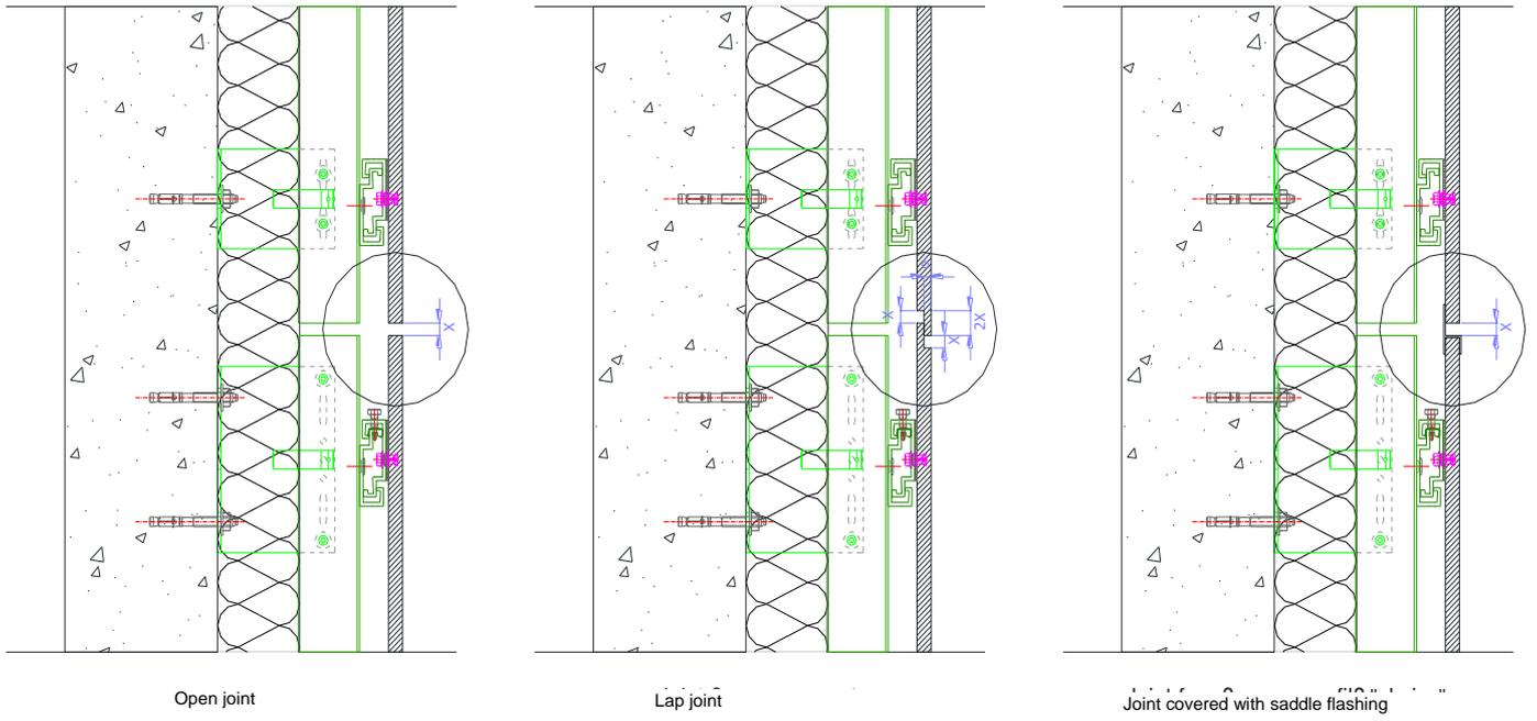
**Figure 12 - Various treatments of horizontal and vertical joint**
