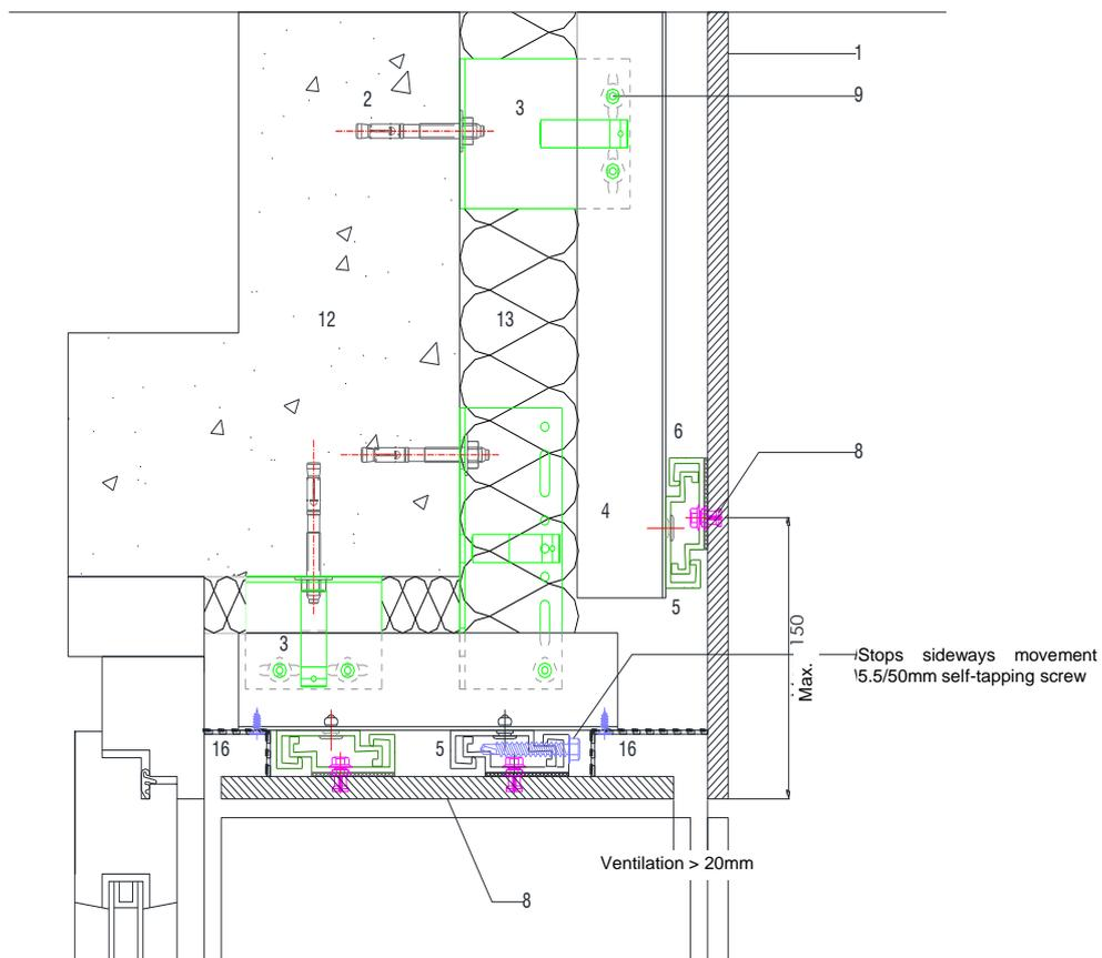
**Figure 20 - Window lintel with HI-MACS® panel cladding**
