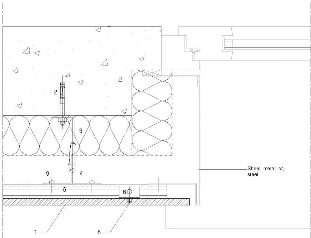
**Figure 21 - Window board with sheet metal cladding**
