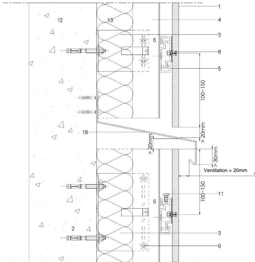
**Figure 15 - Horizontal compartmentalisation of air gap**
