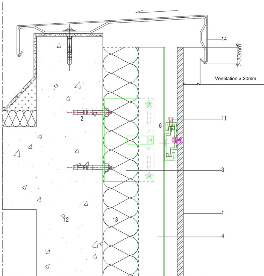
**Figure 13 - Parapet cap**
