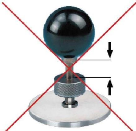
You cannot push the gauge down to the base section without the thickness wedge.
