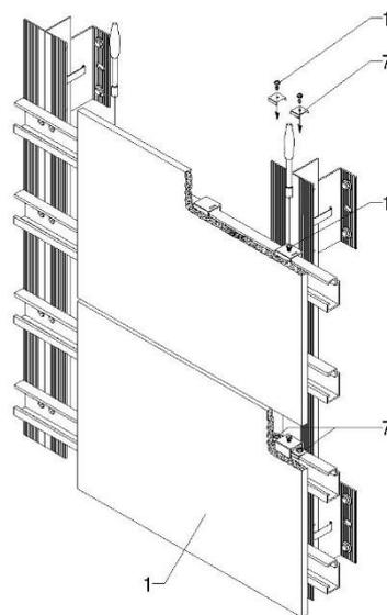
Figure 1 – Panel and metal frame assembly functional diagram
