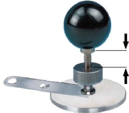
2 - Place the thickness wedge between the panel and base section of the control gauge. The machined hole is compliant if you cannot push the gauge down to the base section.
