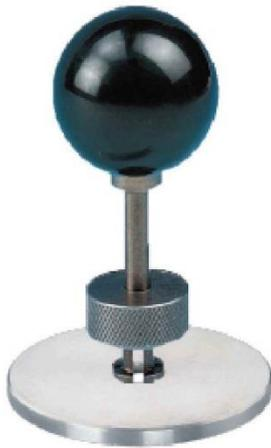
Insert the base section of the control gauge in the machined hole that holds the insert.
