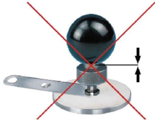
You cannot push the gauge down to the base section with the thickness wedge.
